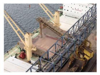
Figure 18 – Vertical Ship Loader Photo Credit: Quorum Corp.
