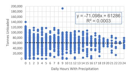
Figure 22 – Daily Tonnes Unloaded from Railcars vs Hours with Precipitation
