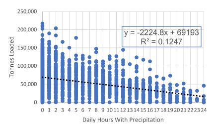
Figure 21 – Daily Tonnes Loaded onto Vessels vs Hours with Precipitation
