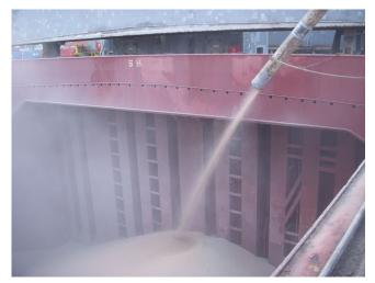
Figure 19 – Marine Spout Ship Loader Photo Credit: Quorum Corp.
