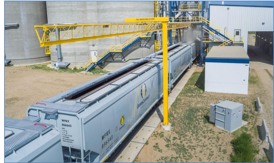
A string of next-generation covered-hopper cars is seen entering the load-out area of the new GrainsConnect facility located in Maymont, Saskatchewan, in 2018. The company was among the first to construct an all-new, state-of-the-art network to exploit the efficiencies inherent in moving unit trains of high-capacity railcars through the grain supply chain. (Image courtesy of GrainsConnect Canada)
