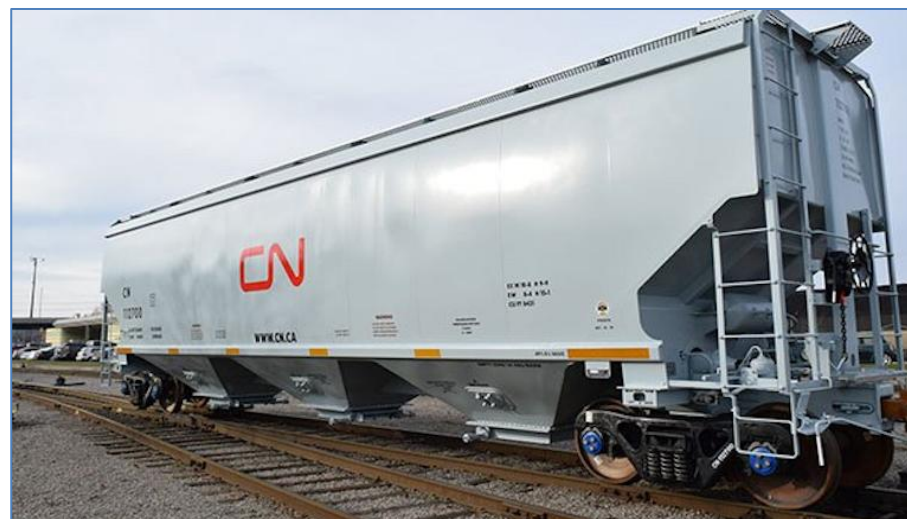
A new covered-hopper car is seen at the National Steel Car facility in Hamilton, Ontario, following its construction in 2019. This was but one of the first in a combined multi-year acquisition of some 11,900 higher-capacity railcars by CN and CPKC, which were intended to replace the aging fleet of cylindrical hoppers cars that had been supplied by the Government of Canada for the movement of Western Canadian grain. (Image courtesy of National Steel Car)
