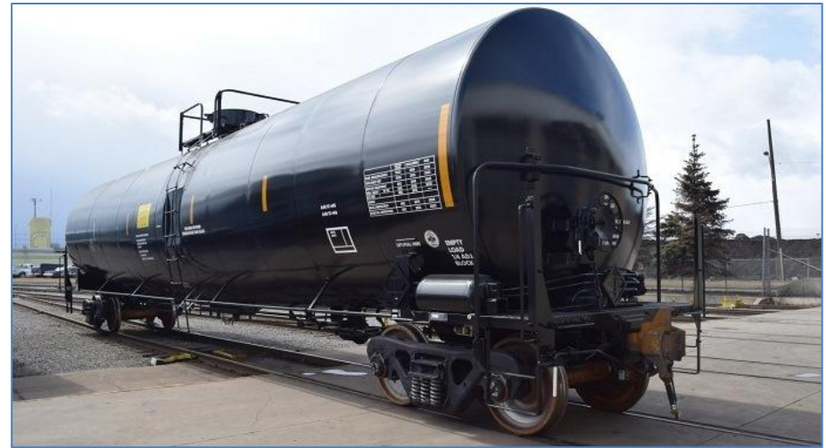
A 25,500-gallon general-purpose tank car is seen following its construction at the National Steel Car facility in Hamilton, Ontario. In addition to petroleum and chemicals, railcars such as these are used to carry a variety of food-grade products, including canola and other vegetable oils. (Image courtesy of National Steel Car)
